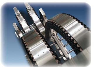
Description of Operation: This machine receives parts from the conveyor at random spacing and captures them on a continuous moving set of gripper chains. They are then lowered (or raised, depending on the configuration) to a discharge point where they are transferred onto a take-away conveyor.
