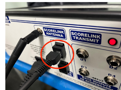
Back of console where handheld device plugs into either of the RJ-45 ports
