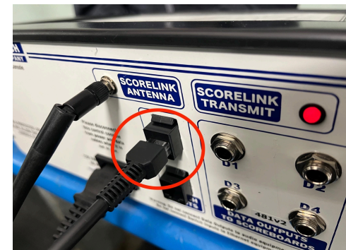
Back of console where handheld device plugs into either of the RJ-45 ports
